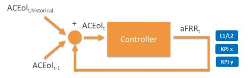
Figure 19: Visual representation of the LFC controller
