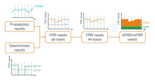
Figure 3: Calculation process of the FRR/aFRR/mFRR needs
