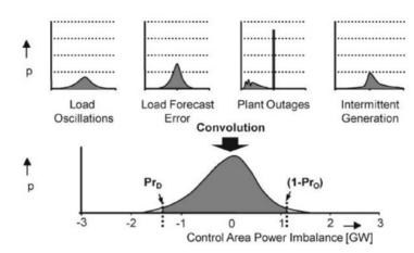
Figure 12: Illustration of the Graf-Haubrich method
